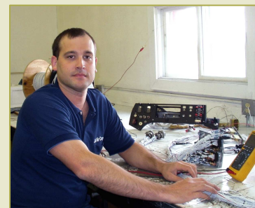
Avionics manager, Joe Megna Jr. building a wire harness for an avionic stack. Much of an install package can be pre-wired for reduced downtime.
