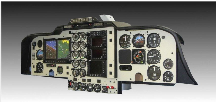
Mike Lavers' custom instrument panel for his -10 "K" model (note the angled avionic stack, relocated autopilot mode selector). The G600 PFD is centered for better visibility for the pilot.
